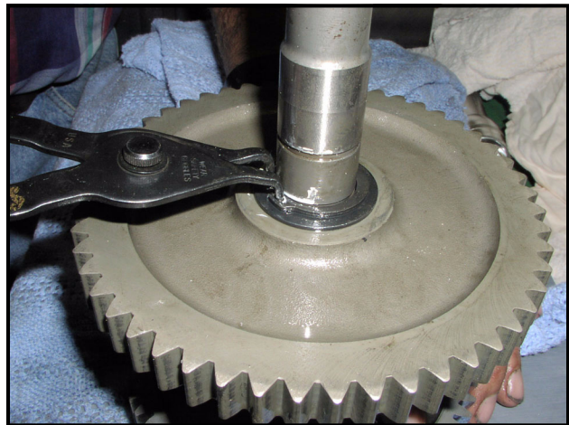
Figure 8-36 Snap Ring and Washer on Chain Sprocket
