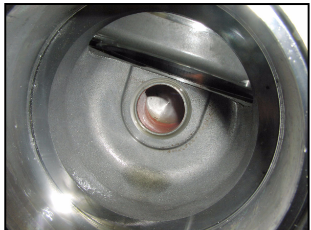
Figure 9-32 Inspect Pinion Gear Shaft Bushing
