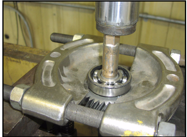
Figure 8-31 Remove Small Helical Gear Bearing
