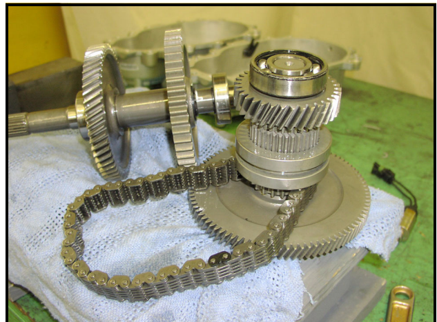
Figure 8-19 Separate Intermediate and Output Gear Assemblies
