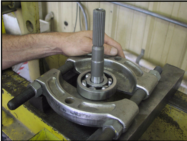
Figure 8-20 Remove Old Input Shaft Bearing
