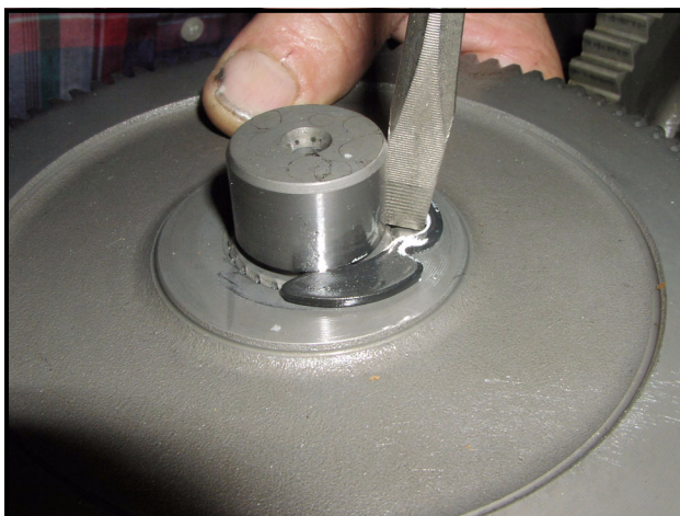
Figure 8-24 E-Clip and Washer on Large Helical
