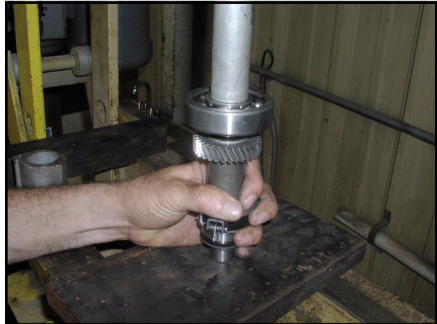
Figure 8-21 Press-On New Input Shaft Bearing
