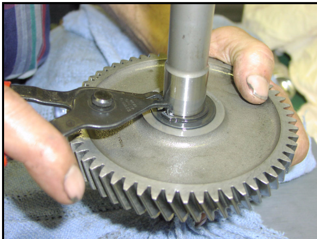
Figure 8-39 Remove Snap Ring and Flat Washer
