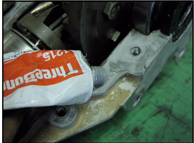
Figure 10-24 Apply ThreeBond 1215 Compound
