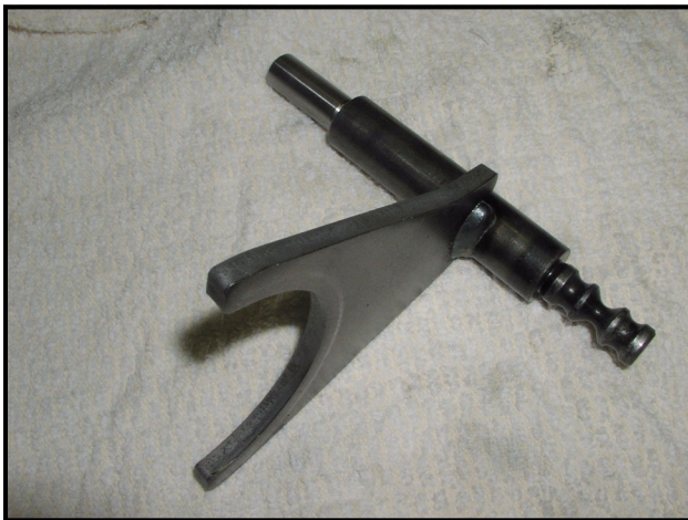
Figure 8-14 Engagement Gear Fork
