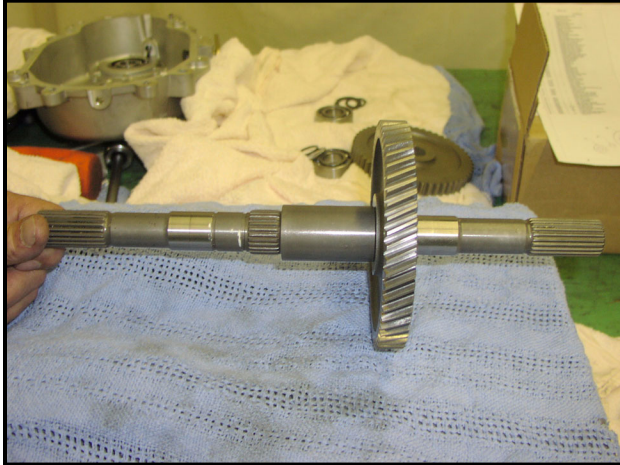
Figure 8-47 Slide Large Helical Gear onto Shaft
