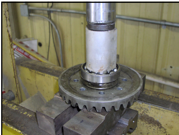
Figure 10-13 Press Bearing onto the Ring Gear
