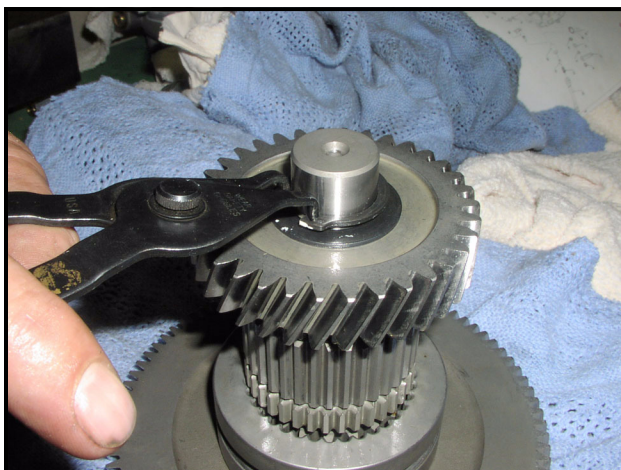
Figure 8-73 Snap Ring on Small Helical Gear
