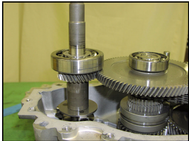
Figure 8-9 Input Shaft, Gear and Governor Assembly
