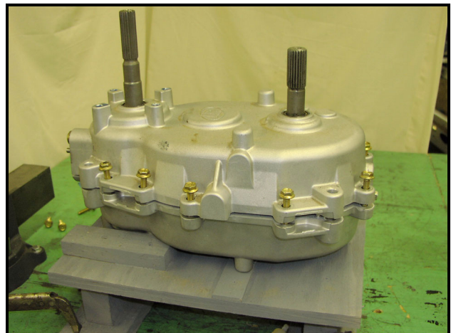
Figure 8-5 Remove Case Bolts
