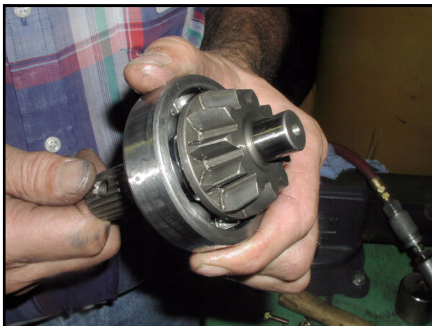
Figure 9-31 Inspect Pinion Gear Bearing
