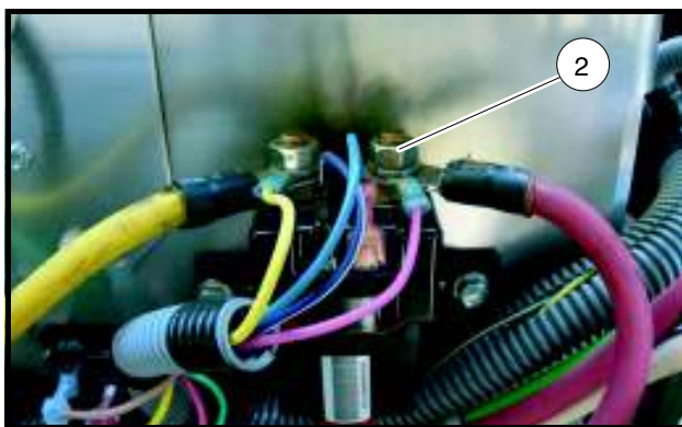
Figure 11-16 Test Continuity: Pink Wire on Solenoid Post
