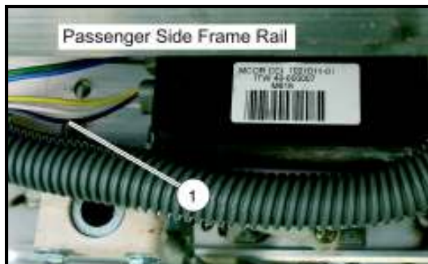
Figure 11-11 Test MCOR: Purple/White Wire (+)
