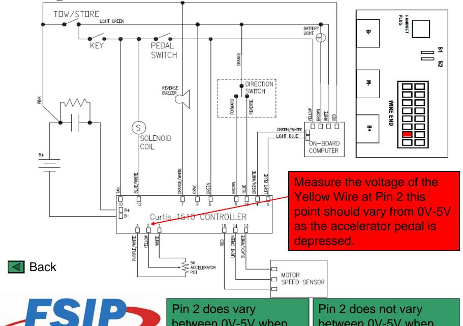
between 0V-5V when moving the accelerator pedal.
