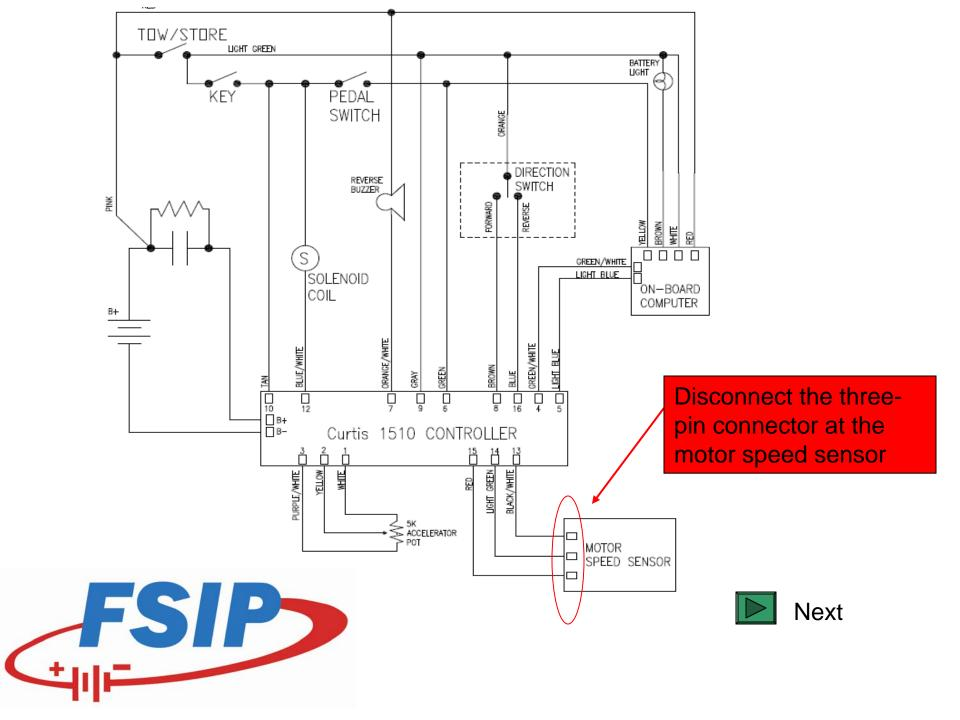
Using a digital voltmeter measure the voltages of the following pins of the motor speed sensor wires.
