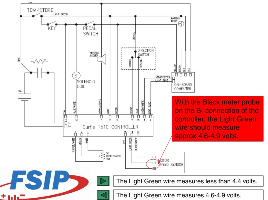
Verify the continuity of the Light Green wire from pin 14 of the controllers 16 pin connector to the three pin connector at the motor speed sensor and replace wire if necessary.
