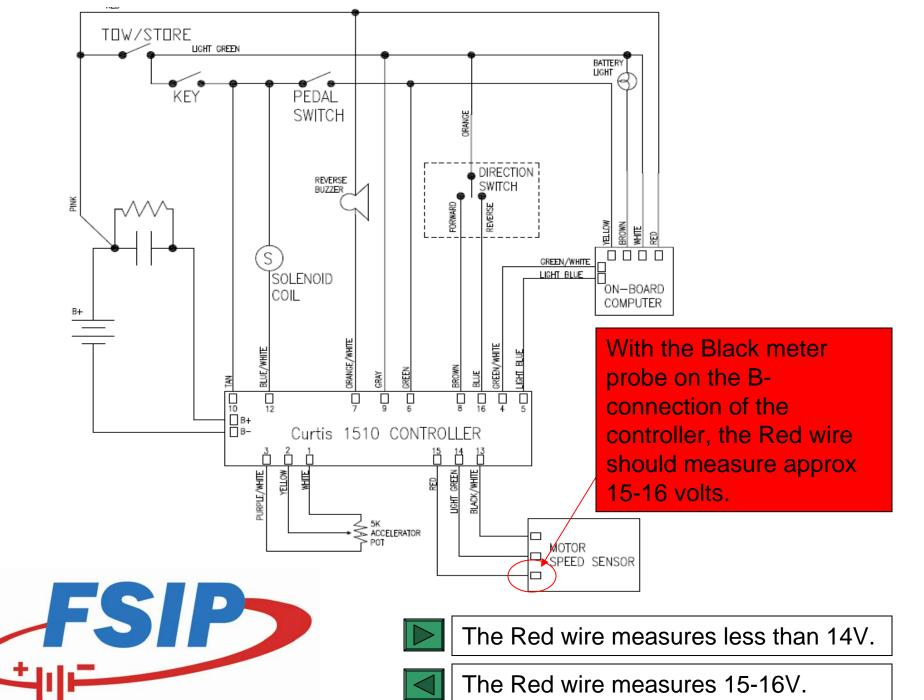
Verify the continuity of the Red wire from pin 15 of the controllers 16 pin connector to the three pin connector at the motor speed sensor and replace wire if necessary.
