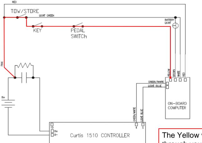
The Yellow wire is supplied through your Run/Tow switch, Key switch, and your Pedal switch verify this connection.
