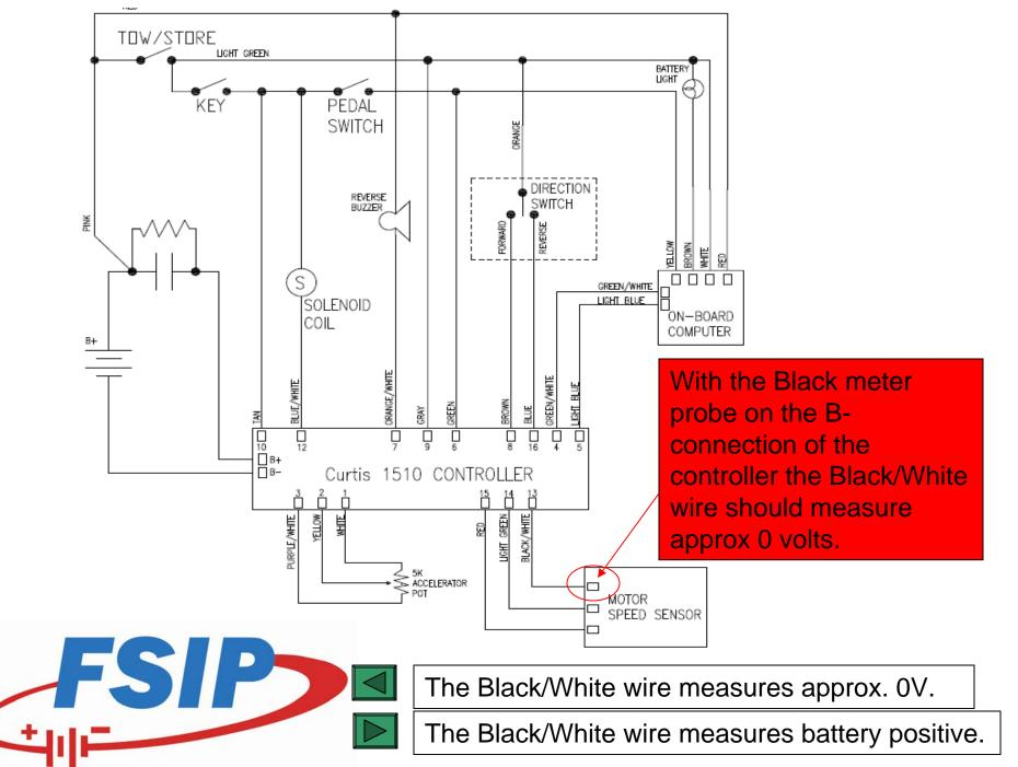
Verify the continuity of the Black/White wire from pin 13 of the controllers 16 pin connector to the three pin connector at the motor speed sensor and replace wire if necessary.
